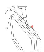
Secure with the top screw so that the panel cannot be removed from the backplate.
